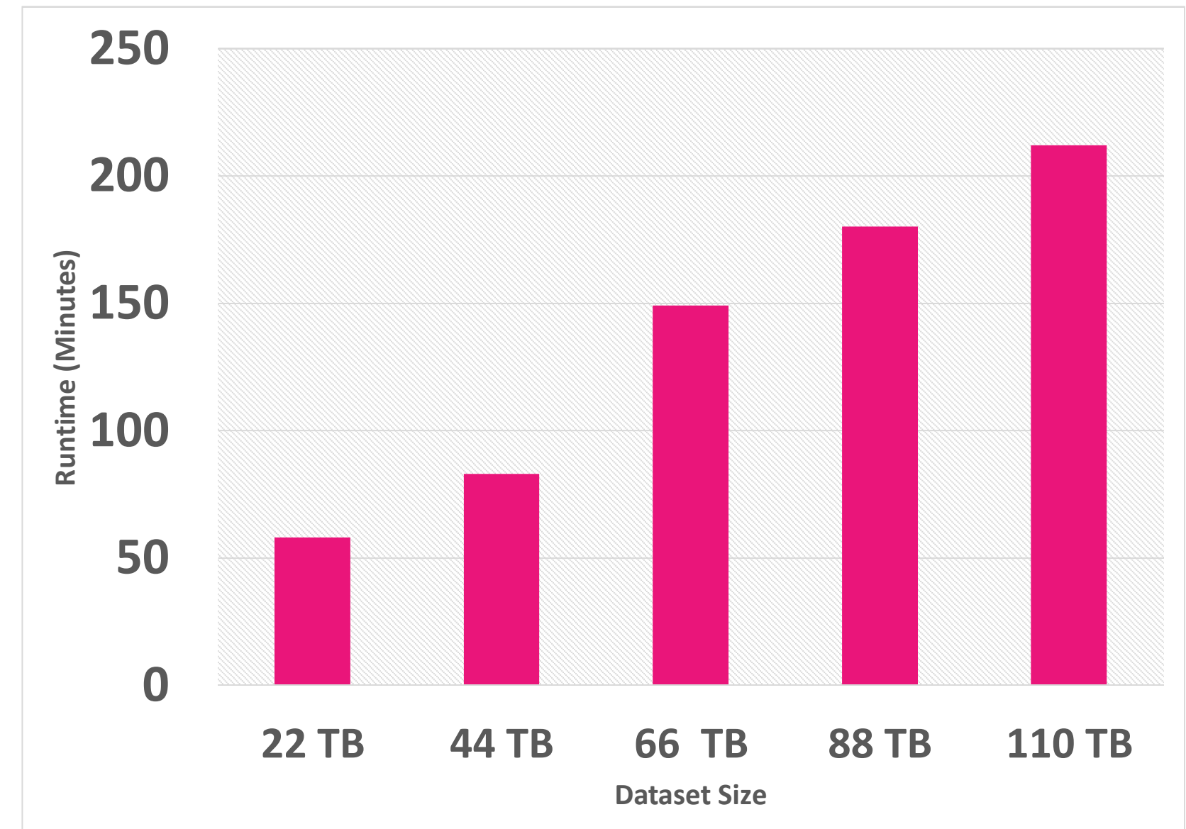
Graph 1: Runtime performance in minutes for different input size with 407 Spark executors, 2 cores per Spark executor, 7 GB per Spark executor. The “readAhead” connector buffer is set to 32 MB.
